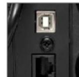
Built-in interface port for remote monitoring of UPS operating modes
