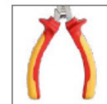
Double-layer plastisol insulated handles. Rated for live work up to 1000 V. Stops on the handles prevent sparks from jumping onto the hand and prevent the hand from slipping into the work area
